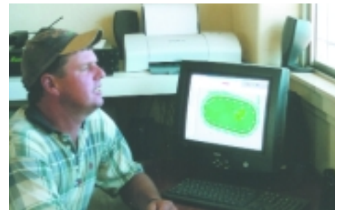
The Rain Bird Site Control system includes a graphic overlay of the race course showing actual sprinkler and zone locations.
