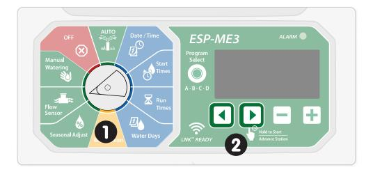
3. You will now be able to turn off flow sensor by station. Using the left and right arrow buttons to navigate between stations and the + and - buttons to turn the sensor on/ off.
