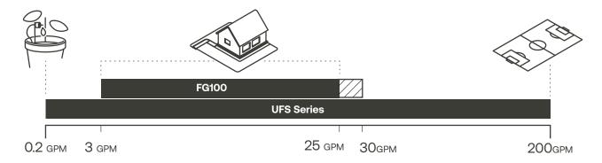
High-output rotors (such as those used on sports fields) may exceed the recommended flow rate of this device. High-efficiency emitters like drip irrigation and high-efficiency spray nozzles may have flow rates that fall below the minimum operating flow of the FG100.
