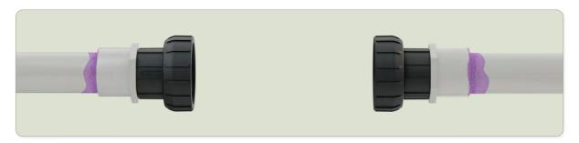
6. Make sure the red filter basket is installed on the upstream side of the flow sensor. Check that the green o-rings are installed properly in the channels on each side of the flow sensor as shown before attaching the flow sensor.
