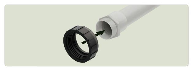
5. Make sure that the pipes are aligned properly to avoid cross-threading.
