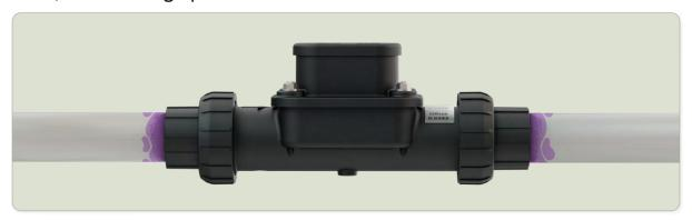
**1.** Measure and cut a 7 1/16" (183mm) section of pipe to accommodate the FG100, Couplings and PVC fitting. If your installation includes an <u>in-line valve</u> then you will need to calculate the length of the section to remove based on your components. Make sure the cut is clean, free from burrs, and straight.
