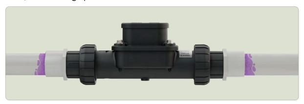
**1.** Measure and cut a 7 1/16" (189mm) section of pipe to accommodate the FG100, Couplings and PVC fitting. If your installation includes an <u>in-line valve</u> then you will need to calculate the length of the section to remove based on your components. Make sure the cut is clean, free from burrs, and straight.
