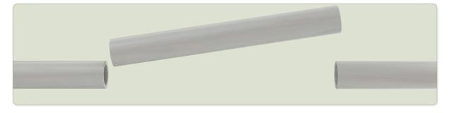
2. Glue the 1" male threaded union fittings to the cut ends of the pipe using PVC cement.
