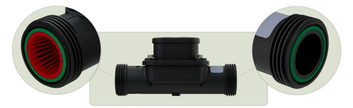
7. Align the FG100 with the union fittings ensuring that the "Flow" arrow is facing in the same direction that water will flow through your system.
