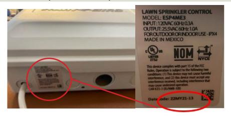
In general, Rain Bird controllers have a date code on the bottom of the external case (if they come mounted in one) and another date code on the back of the main panel.
