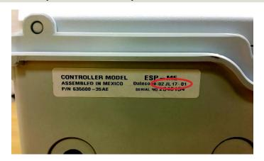
In general, Rain Bird controllers have a date code on the bottom of the external case (if they come mounted in one) and another date code on the back of the main panel.
