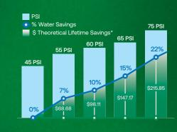
The savings reaped per rotor can be multiplied across an entire system, resulting in significant differences financially and in gallons of water used.
