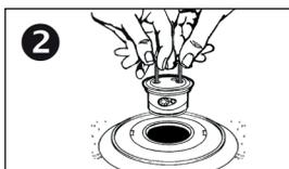
**3** Press the replacement nozzle assembly into the nozzle housing, making sure the nozzle front is flush with the outside of the housing.
