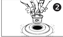
2 Grasp the nozzle housing screws and lift up to separate the nozzle housing from the internal.
