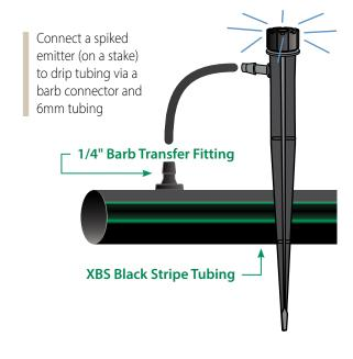
The SQ series nozzle or any 1032 Thread emitter can be placed on a PolyFlex Riser Stake and connected to drip tubing.
