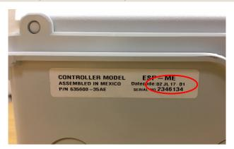
In general, Rain Bird controllers have a date code on the bottom of the external case (if they come mounted in one) and another date code on the back of the main panel.
