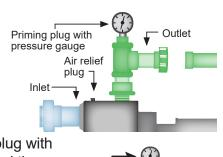
Remove priming plug with pressure gauge and the air relief plug on top of pump.
