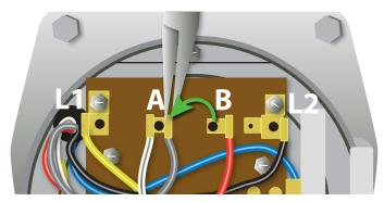
For 115 V service, remove the motor cover and change the following wires on the terminal board:
