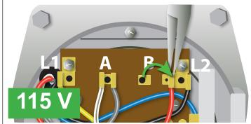
b. Pull the red wire with the female flag connector from the "B" terminal. Place it to the right on the L2 terminal space post.
