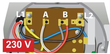
The motor of this pump is dual voltage and can run on either 115 V or 230 V. This pump is pre-set in the factory to run at 230 V.
