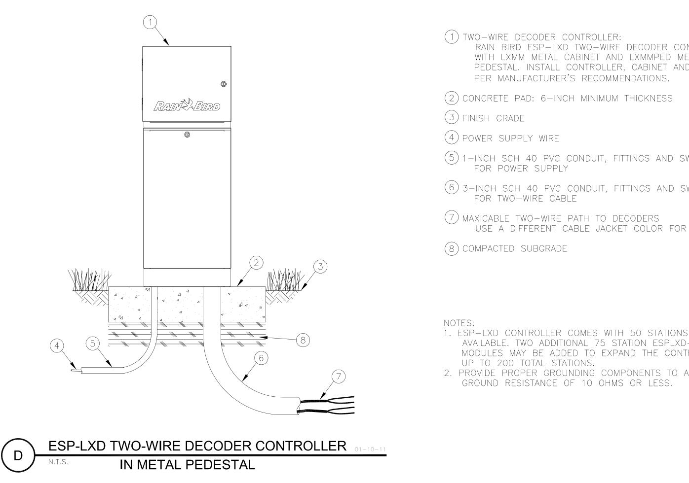
RAIN BIRD ESP-LXD TWO-WIRE DECODER CONTROLLER WITH LXMM METAL CABINET AND LXMMPED METAL PEDESTAL. INSTALL CONTROLLER, CABINET AND PEDESTAL
