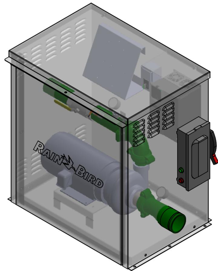
1. CLOSE-COUPLED, HORIZONTAL END-SUCTION PUMP WITH BRONZE IMPELLER AND TYPE 21 BUNA-N MECHANICAL SEAL FOR LONG PUMP LIFE.
