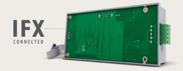
1. The IFX Satellite Board is standard in all Rain Bird PAR+ES Satellites manufactured after 12/22/19 and is compatible with all PAR+ES, PAR+ and MSC+ Satellites. To add the IC System to an ICI+LINK with LINK Satellite System, simply install an ICI+Two-Driver Board (sold separately), connect the MAXI Cable to the interface, then add IC Rotors, IC Valves or IC CONNECT devices to the MAXI Cable. 2. Requires ICI+LINK with LINK Satellites.
