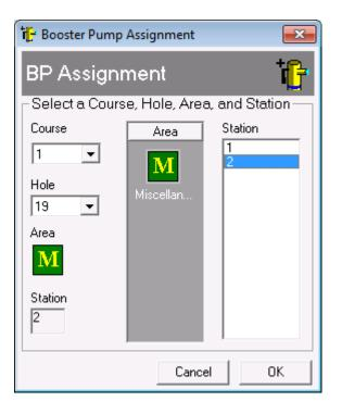
12. Assign related branches, flow zones and stations to the booster pump using the same method as creating a new Flo-Manager<sup>®</sup> tree.
