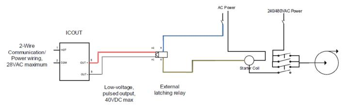
Figure 1. IC-OUT Controlling a Latching Relay in a Pump Starter Coil Application
