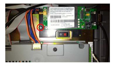
5. Secure the radio/modem in place using a drill to drive the two 3/16 6-20 thread self-tapping screws into the PAR+ES metal bracket through the plastic mount plate on either side of the power switch. Place the paper slip over the top of the PIB to prevent metal shavings from entering the PIB while drilling.
