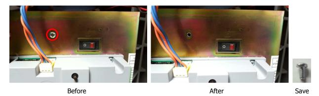
2. Install 4 Hex Standoffs on the bottom of the LINK900 radio/modem assembly.
