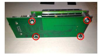
3. Secure the mounting plate to the radio/modem assembly by threading the two 3/16" 4-40 thread screws into the standoffs through the plate. Orient the plate onto the radio/modem according to this picture.
