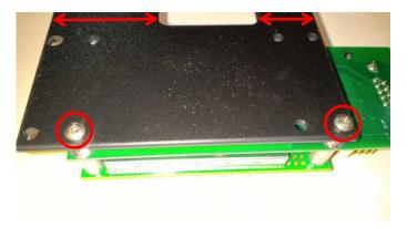
4. Use the screw saved in step 1 to attach the radio/modem to the PAR+ES controller above the power switch.
