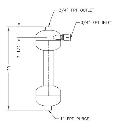
FLOW RATE: 10 - 20 GPM.
