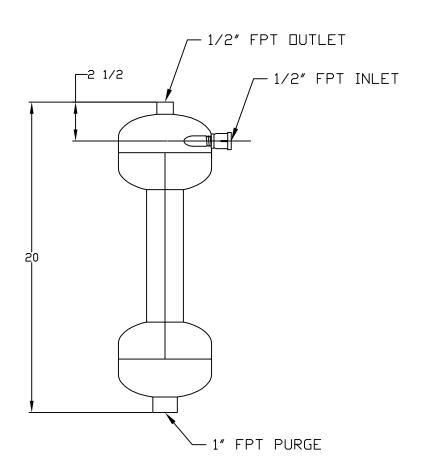
FLOW RATE: 4 - 10 GPM, PRESSURE RATING: 150 PSI, SHIPPING WEIGHT: 13LBS,
