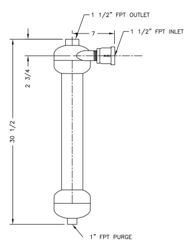
FLOW RATE: 38 - 79 GPM.
