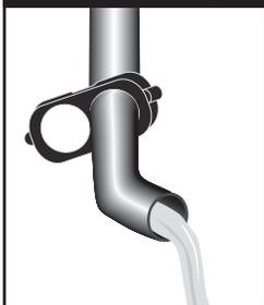
Remove end closures and flush out the system until the water runs clear. Perform maintenance 1-2 times a year.
