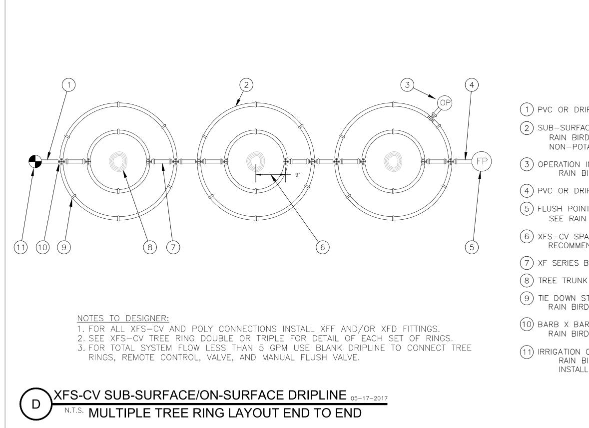
XFS-CV Sub-Surface On-Surface Dripline Multiple Tree Ring Layout End To End
