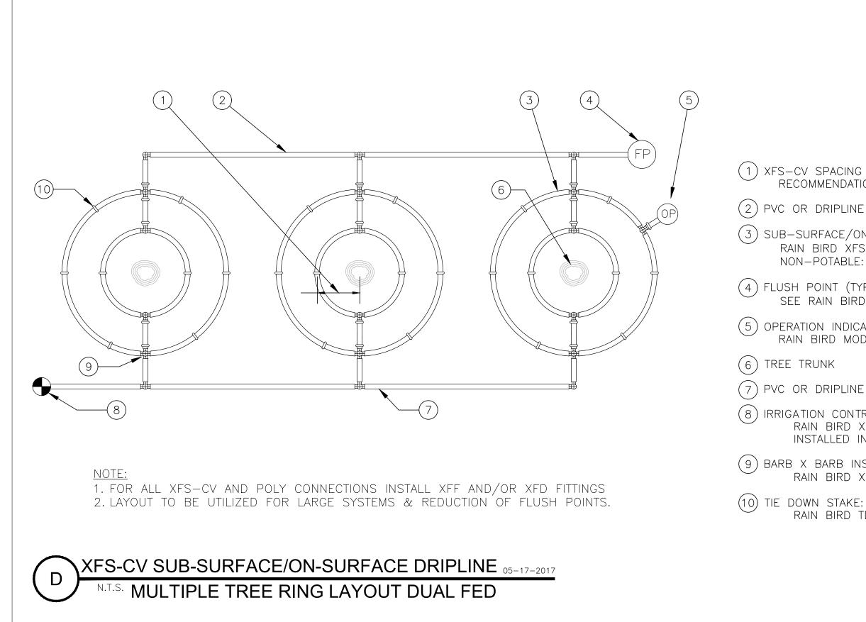
XFS-CV Sub-Surface On-Surface Dripline Multiple Tree Ring Layout Dual Fed
