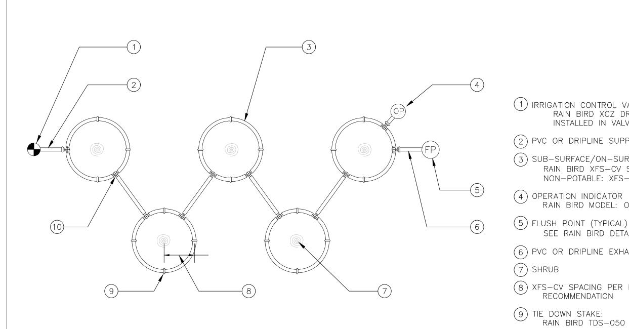
NOTE: 1. FOR ALL XFS-CV AND POLY CONNECTIONS INSTALL XFF AND/OR XFD FITTINGS.
