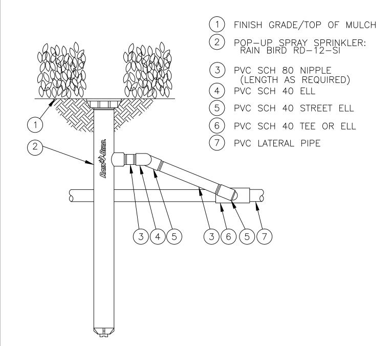
HE-VAN NOZZLE MPR NOZZLE ROTARY NOZZLE SQ NOZZLE U-SERIES NOZZLE VAN NOZZLE <u>OPTION</u> NON-POTABLE CAP
