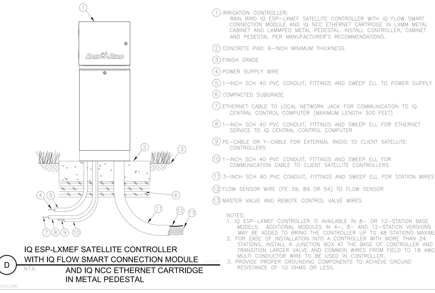
MODELS. ADDITIONAL MODULES IN 4-, 8- AND 12-STATION VERSIONS MAY BE ADDED TO BRING THE CONTROLLER UP TO 48 STATIONS MAXIMUM. STATIONS, INSTALL A JUNCTION BOX AT THE BASE OF CONTROLLER AND TRANSITION LARGER VALVE AND COMMON WIRES FROM FIELD TO 18 AWG
