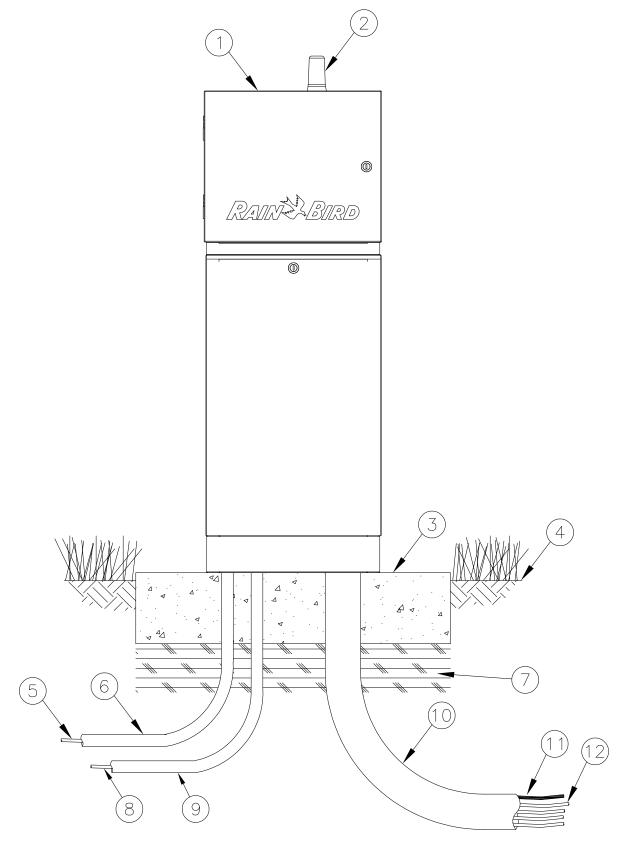
IQ ESP-LXMEF SATELLITE CONTROLLER WITH IQ FLOW SMART CONNECTION MODULE
