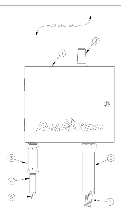
IRRIGATION CONTROLLER: RAIN BIRD IQ ESP-LXME SATELLITE CONTROLLER WITH IQ NCC GPRS CARTRIDGE IN LXMM METAL CABINET WITH OUTSIDE
