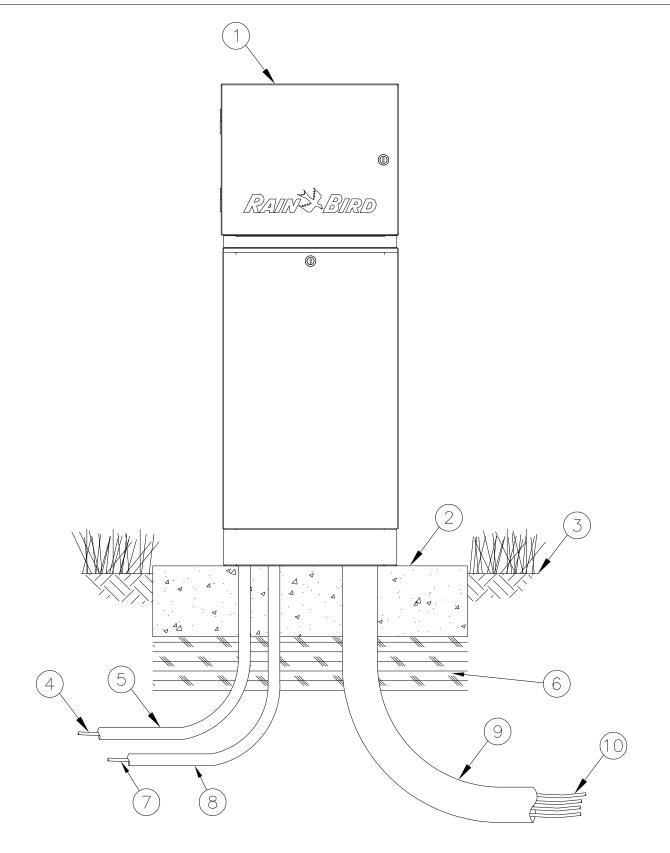
IQ ESP-LXME SATELLITE CONTROLLER WITH IQ NCC RS232 CARTRIDGE
