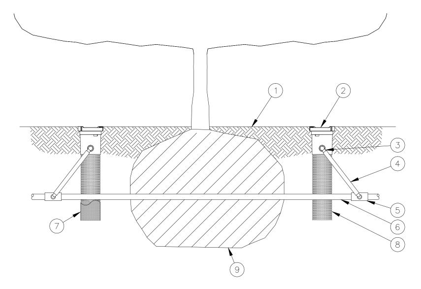
FINISH GRADE/TOP OF MULCH RAIN BIRD SBÉ-050 PVC SCH 40 TEE OR EL (5) PVC OR POLYETHYLENE LATERAL PIPE (8) PLANT ROOT BALL 9)
