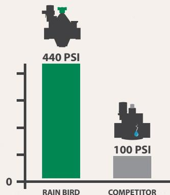
If high water pressure strikes, you need to be prepared for the worst-case scenario. For the Burst Test, we ramped up the pressure as high as it could go. We did the same for the valves of a leading competitor. The results were telling. While the competition exhibited body-to-bonnet leaks under pressures as low as 100 psi (6.9 bar), the PGA valve held strong, even at 440 psi (30 bar).
