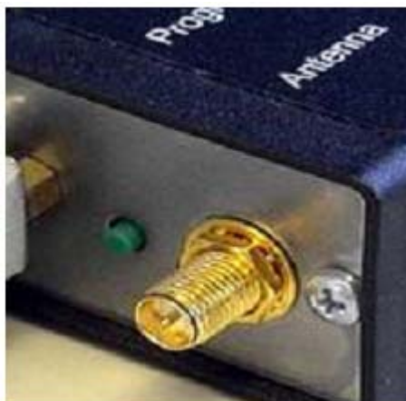
FIGURE 8 The connector marked Antenna on an RFXX-series radio is where the antennas attach.
