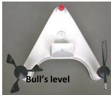
FIGURE 14 Bull's Level on top of the weather station
