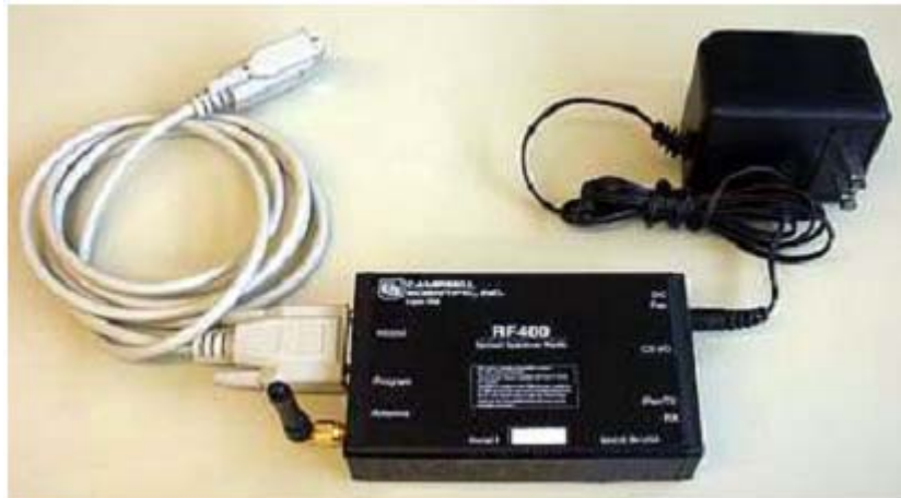
FIGURE 9 Radio connections. The serial cable (left) connects to the port marked RS232 and the AC adapter connects to the port marked DC PWR input.
