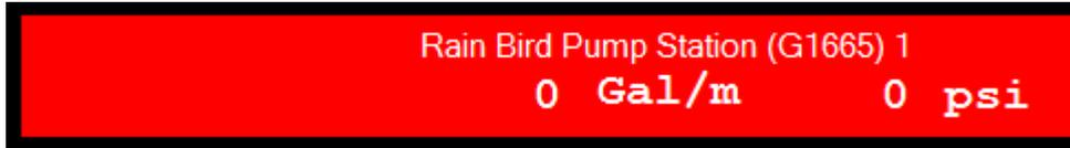
To distinguish between a communication error and pump station alarm, refer to the Pump Manager 2 main window, selecting the error pump station from the Pump Stations list.
