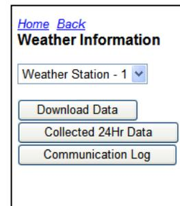
**Download Data:** This button will cause SmartWeather at your central control to communicate with the weather station and retrieve the most current weather data. When you depress [Download Data](#) button, you will receive a message from the Rain Bird MI Series Mobile Controllers server indicating the request was received and
