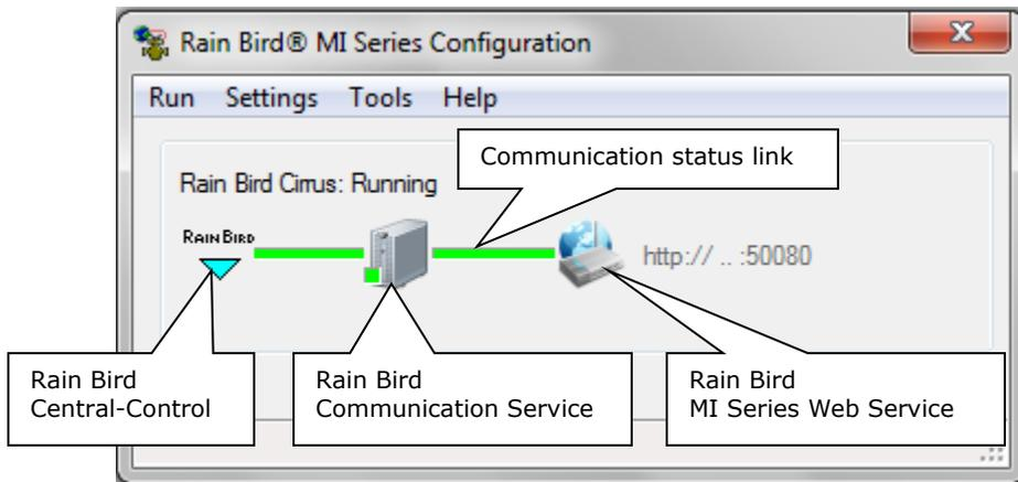
Rain Bird Communication Service is a bridge between the central-control app and MI Series Web Service. A little square indicator at Rain Bird Communication Service shows the service status. If the indicator is green, the Rain Bird communication service is functioning correctly. If the indicator became red, the service is not working. Please refer to [Communication Service Problems](#) at the [Troubleshooting](#) chapter that help figure out problems. Two green line-bars show communications
