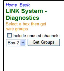
LINK diagnostics are a measure of radio performance. LINK systems continuously check radio status when the central control is running. The diagnostic is the ratio of calls to and responses from each satellite expressed as a percentage. 100% is perfect communication, 0% would be no communication. The diagnostics is tagged as Pass, Check or Fail depending on the percentage.
