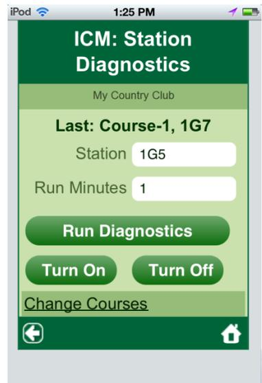
“Run Minutes”, for example one minute. Then click **“Turn On”** button to see if the station can be turn on or not. After the station is on, click **“Turn Off”** button to see if the station can be turn off or not.
