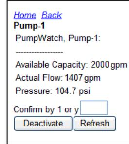
Similarly, Actual Flow is the real-time discharge rate from the pump station. The Flow Rate and pressure shown on the SmartPump data page are the same as the Flow and Pressure windows at the bottom of the Front Office of your central control.
