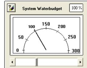
The Rain Bird MI Series Mobile Controllers Water Saver screen is shown here. The top portion of the screen is used to set a System Waterbudget. Enter the percentage desired in the box provided then select the  button to update the setting in your central control.
