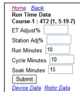
The data pages can also be edited. When edits are made with Rain Bird MI Series Mobile Controllers, the central control database is immediately updated and the new settings are in effect for the next irrigation cycle. The Run Time Data page includes
