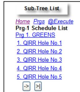
The picture on the right is the QuickMethod view. The QuickMethod allows you to do everything the Tree List does with almost no clicking, selecting or scrolling. Using a special set of command codes (see command code chapter earlier in this document) this simple control panel is the only screen you need to use Rain Bird MI Series Mobile Controllers.
