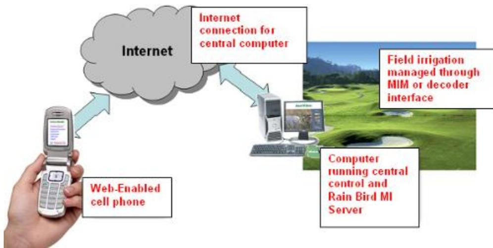
Rain Bird MI Series Mobile Controllers utilize a server running on your central control computer. A remote Web browser such as the micro-browser commonly found on newer cell phones is then used to contact that server and remotely operate your central control.
