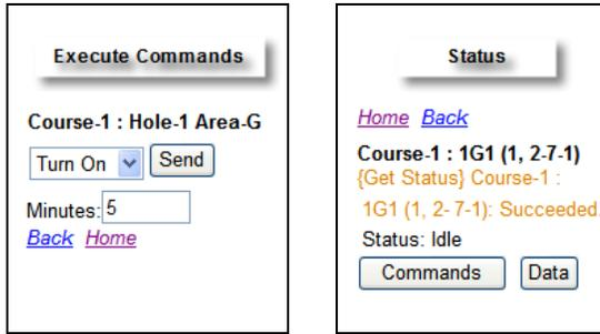
The [@Execute](#) version is a control panel used to perform area level commands. Area level commands include those shown to the right.
