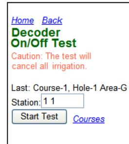
To initiate the Decoder On/Off test, select “Decoder Diags” from the Diagnostics Page then select [On/Off Test](#) from the diagnostic selection screen. This brings up the On/Off Test control panel shown here.
