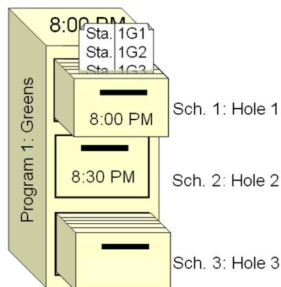
Notice the Program is set to run at 8:00 pm (2000). The schedules for Hole 1 is set to start at 8:00 pm (2000), the schedule for Hole 2 is set to start at 8:30 pm (2030) and the schedule for Hole 3 has no start time. In Rain Bird systems, schedules without a start time (the default) assume the start time of the program – so in this case, the start time for schedule 3 is 8:00 pm (2000).
