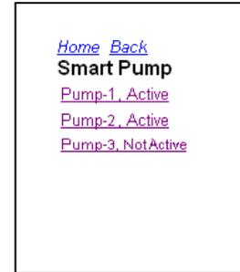
With SmartPump, the central always knows the current pump station capacity, the current station discharge rate and the current system pressure. In Rain Bird MI Series Mobile Controllers, the SmartPump link will display current pump station discharge rate, discharge pressure and station capacity. The units of flow are displayed using the settings defined in your central control.
