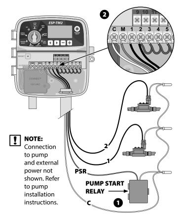
**NOTE:** The ESP-TM2 controller DOES NOT provide power for a pump. The relay must be wired according to manufacturer instructions.
