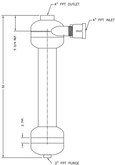
FLOW RATE: 190 - 345 GPM. PRESSURE RATING: 150 PSI. SHIPPING WEIGHT: 120 LBS.
