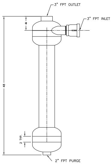
FLOW RATE: 125 - 260 GPM. PRESSURE RATING: 150 PSI. SHIPPING WEIGHT: 120 LBS.
