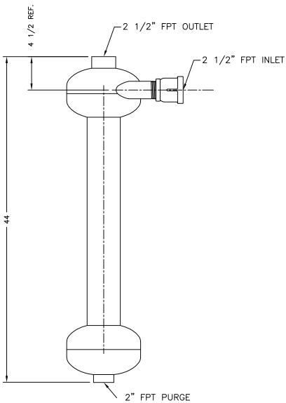
FLOW RATE: 100 - 180 GPM. PRESSURE RATING: 150 PSI. SHIPPING WEIGHT: 55 LBS.
