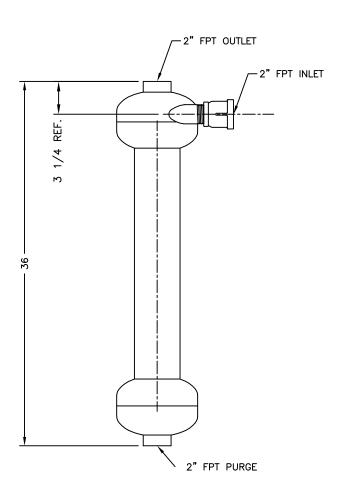
FLOW RATE: 63 - 120 GPM. PRESSURE RATING: 150 PSI. SHIPPING WEIGHT: 44 LBS.
