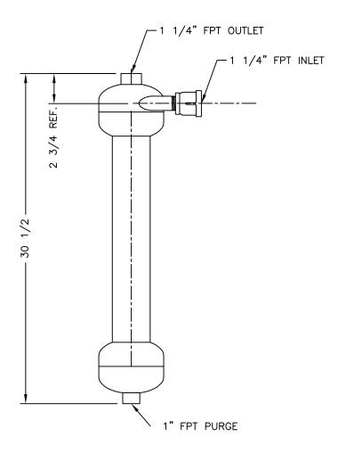
FLOW RATE: 26 - 52 GPM. PRESSURE RATING: 150 PSI. SHIPPING WEIGHT: 26 LBS.
