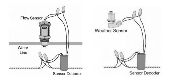
Note: SD-210TURF Sensor Decoders are required for use in U.S. and Canada (60 Hz power). SD210 Sensor Decoders are required for use in the rest of the world (50 Hz power).
