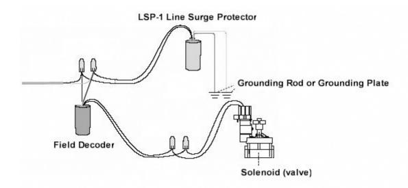
Refer to page 24 of the ESP-LXD 2-Wire Decoder Coontrol System Installation & Troubleshooting Guide for recommended location and quantity of LSP-1 Lightning Surge Protectors.
