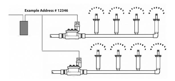
FD-202 Two addresses – each controlling two valves simultaneously
