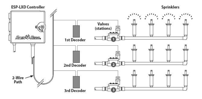
**Typical 2-Wire Decoder to Valve Connections**
