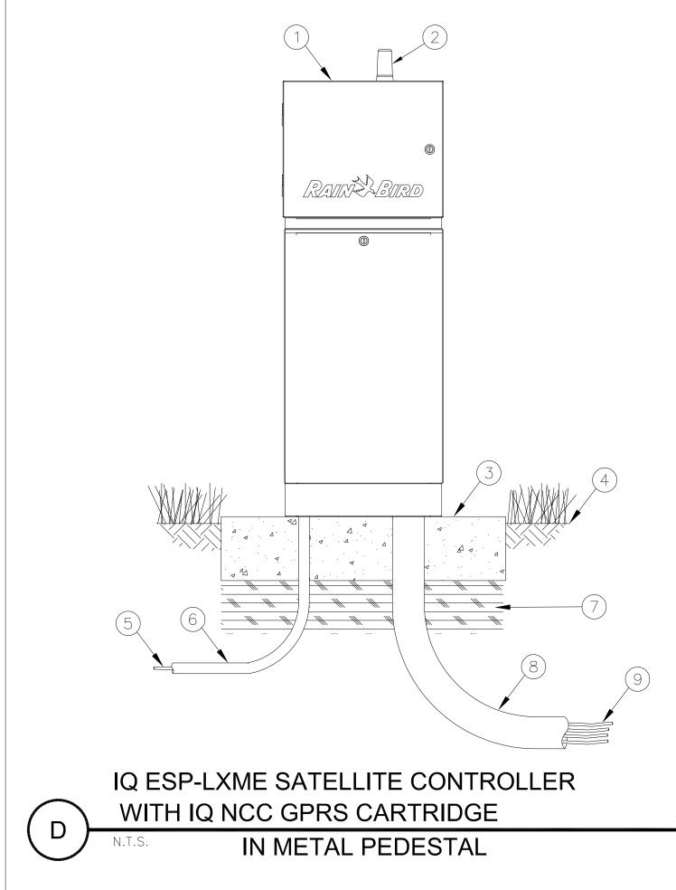
**IRRIGATION CONTROLLER:** RAIN BIRD IQ ESP-LXME SATELLITE CONTROLLER WITH IQ NCC GPRS CARTRIDGE IN LXMM METAL CABINET AND AND PEDESTAL PER MANUFACTURER'S RECOMMENDATIONS.
