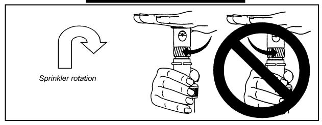
Always turn head in the same direction the sprinkler is rotating. Turning the head against the sprinkler's rotation may damage the sprinkler.
