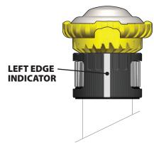
**1.** Align the nozzle to the left most edge of desired coverage area (arc).
