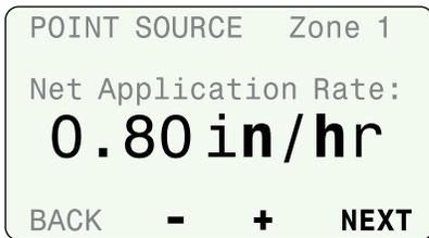
**NOTE:** Increasing the Net Application Rate will decrease irrigation run times, and decreasing the value will increase the run times.
