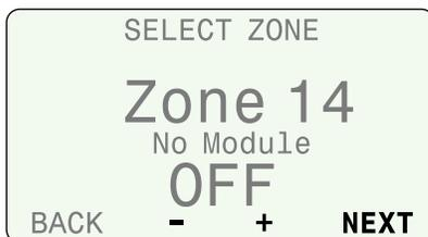
**!** **NOTE:** Station numbering gaps will not prevent the controller from operating properly. It only affects station numbering. During programming when connected to AC power, the controller will skip any unused stations where a module is not installed.
