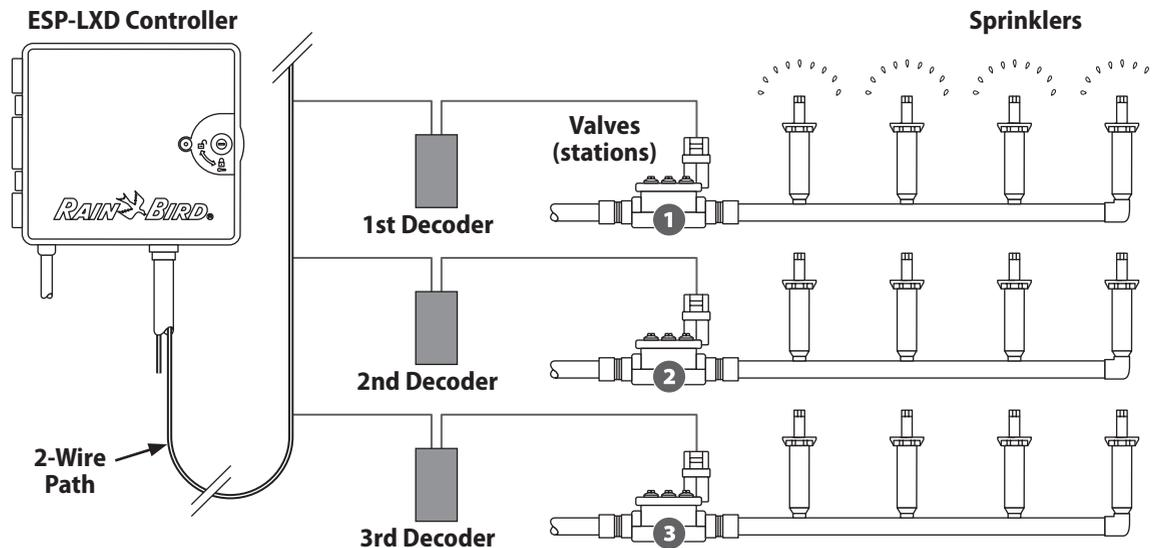
Figure A.4 - Typical Decoder and Valve Operation
