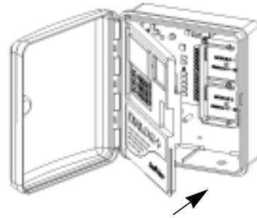
7- Reconnect the 230VAC power supply wires.
