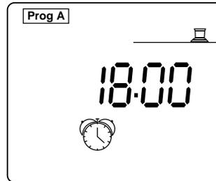
You can repeat the same irrigation cycle up to 8 times a day = 8 start times to meet your water application requirements. At each start time, all the stations assigned to the same program will operate in sequence for the scheduled run times.
