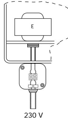
**Note: the controller takes into account the presence of the extension cabinet as soon as the 230VAC power supply is reconnected.**
