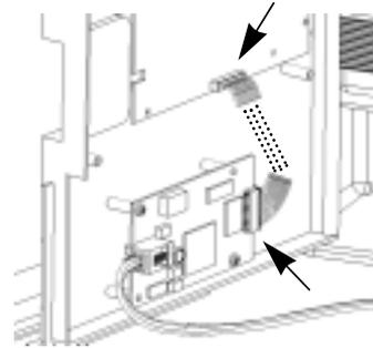
5- Connect the phone line to the modem as shown in diagram 5
