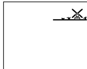
b) There is a blinking cross. You can press +/ON to allow scheduled automatic watering or press -/OFF to prevent it.
