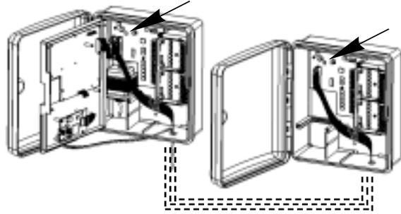
5- Reconnect the 230VAC power supply wires.
