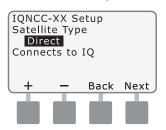
The Setup – Satellite Address screen is displayed. Direct Satellites always have an address of 001; press Next.
