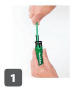
Insert 2-wire cable and press UF Cable Stripper
