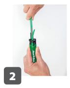
Pull UF Cable Stripper, peeling outer plastic
