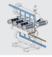
FILTRATION STAGE: As water goes through the discs, particles are projected away due to the cyclone effect, reducing the backflushing frequency.
