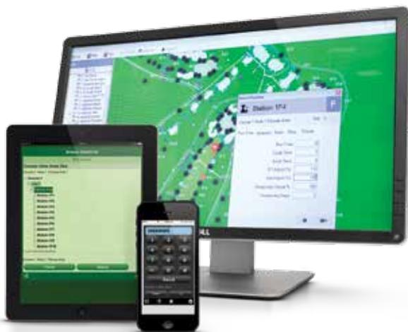
The renovated system included Rain Bird’s MI Series™ Mobile Controller, making it possible for Lukus and his staff to manage irrigation remotely. The MI Series delivers real-time system notifications, advanced diagnostics, and the ability to make instant adjustments via smartphone or tablet. In the office, a 65-inch touchscreen monitor provided another powerful irrigation scheduling and management tool.
