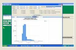
All pump station data, including pressure, flow, manual operations, alarm conditions, water and power usage, is recorded and securely saved on your PC for future analysis and management.
