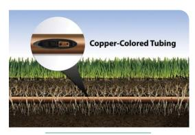
XFS Sub-Surface Dripline with Copper Shield<sup>™</sup> Technology
