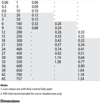
PE-IVM Series Valve Pressure Loss (bar)
